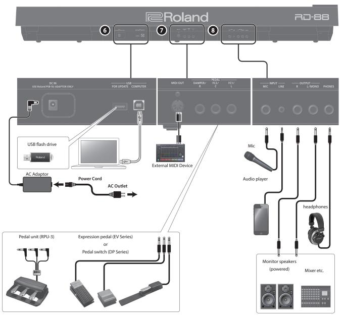
\* To prevent malfunction and equipment failure, always turn down the volume, and turn off all the units before making any connections.
